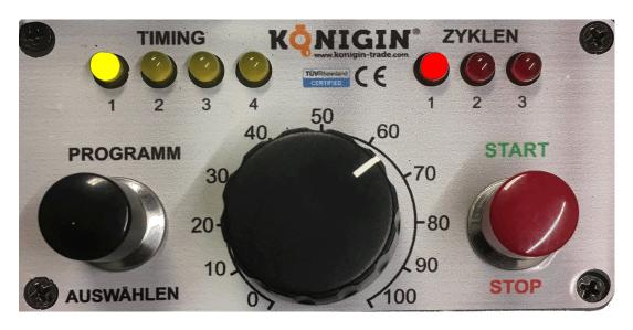
After the Red Start button is pressed the first TIMED CYCLE is started. When the first timed cycle finishes, the machine brakes and slows down (about 10 second) after this it changes the direction of rotation and the second cycle begins. The second period of the speed automatically increase by 30% compared to the first period.
