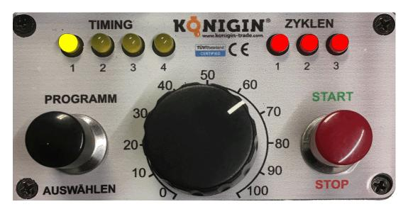
The machine slows down end of the third cycle (approximately 6 seconds) the exactor switches to start position; three short peeping sounds to show this. The red LEDs do not light at this time, one of the yellow LED lights and shows the current selected timing program.
