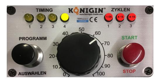
You can leave out the first rotation cycle and run just the second and third rotation cycles. If you do not need a three-cycle rotation, you can set up the exactor to omit the first cycle in the following ways:
