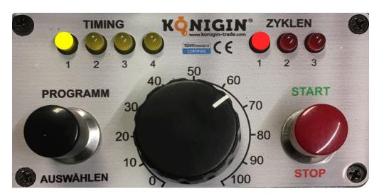
If you press the Red Start button or the black Program button the machine brakes and the rotation slows down and switches to start position. If you press and hold the Red Start button the machine skip the braking period.
