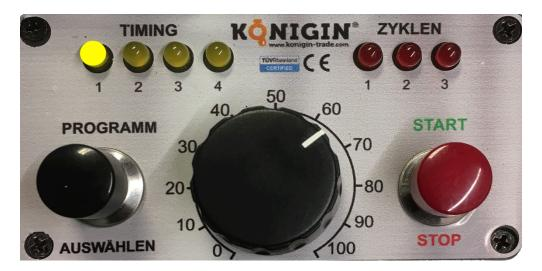
Three short peeping sounds are indicative of root position of the machine .The machine stars and keep working after the green Start button is pressed.
