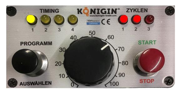
After the braking and stopping the extractor changes of direction the third cycle begins. The speed is not changed automatically. The speed is same in the second and third cycle but you can change the speed with the Speed Control Turning knob.
