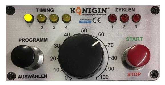
Three short peeping sounds are indicative of start position of the machine. The lighted yellow LED shows the chosen program. The first period is the shortest and slowest one; the fourth period is the longest and fastest one. To start the selected program press the Red Start button!
