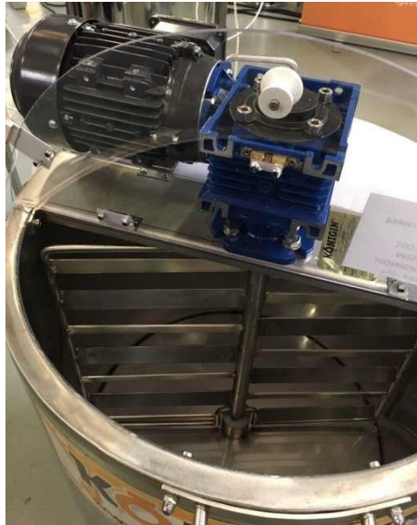
Picture 2. The drive motor with the double-winged mixing paddle
