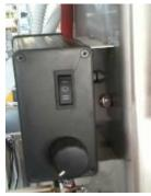
The distance between the knives can be adjusted by moving left hand arm when viewed from the front. If this moves not in the correct distance range, then loosen the screws of the tilting elements provided with bearings on the left ends of the knife axes, and turn the box with the arm to the O position (pushing it forward). Then manually adjust the tilting angle of the knives, and fix the desirable setting by means of the screws.
